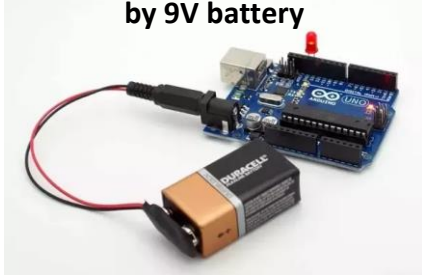
Figure 64, Arduino Uno powered by 9V battery
